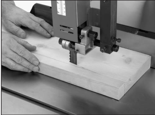
Figure 35. Blade leading away from line of cut.
